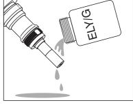
Rinse the sensor head with electrolyte solution.
